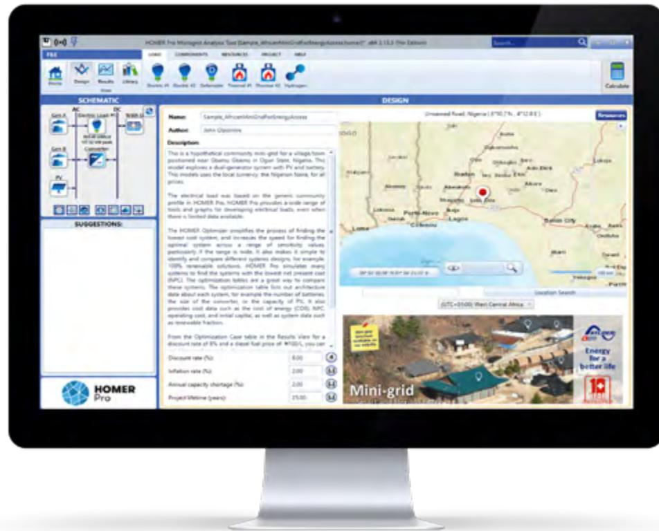
Homer is the most mature design software. It allows for simulations and optimization of mini-grid layouts, as well as sensitivity analyses for the user to learn how external factors (e.g. fuel cost) impact the financial performance of the mini-grid. Homer has an API to integrate with other software (e.g. Odyssey Energy Solutions), as well as add-on modules for different generation technologies.
