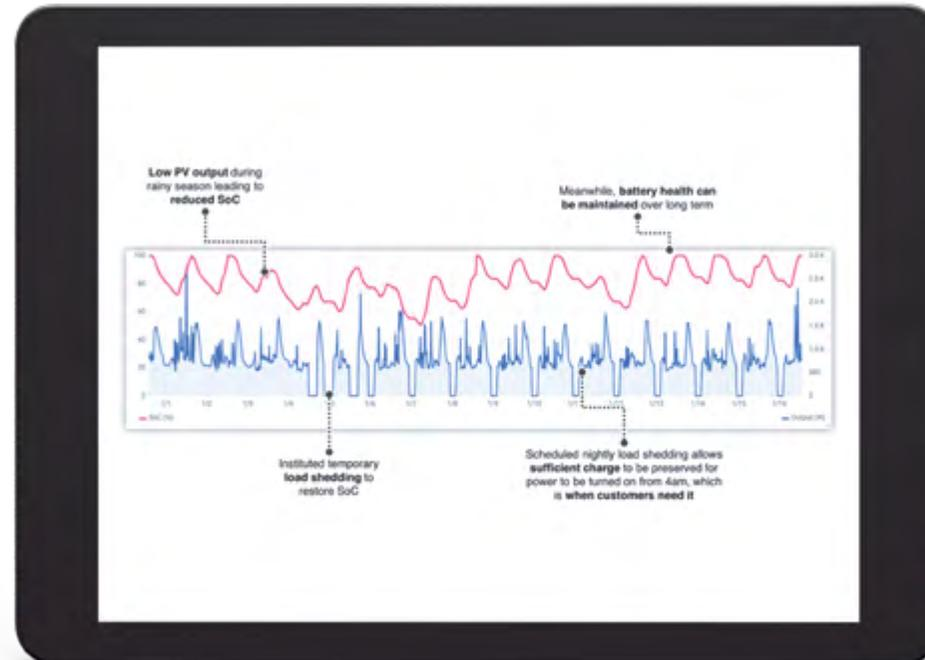
Figure 20 – Example of a system monitoring interface by AMMP<sup>114</sup>
