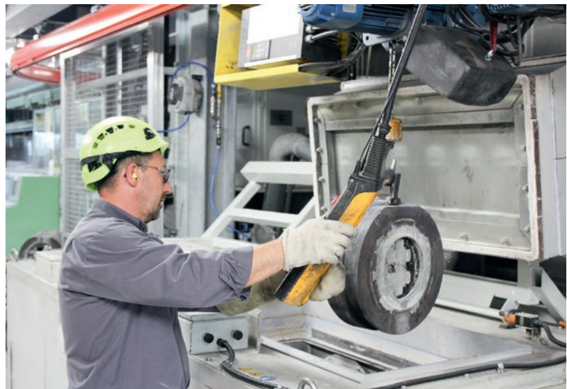
For production to be efficient, the die also need to be heated to a temperature of 470° Celsius, so that there is no difference in temperature between the material and the tool. The image shows how an employee uses a crane to lift a tool out of the induction furnace.
