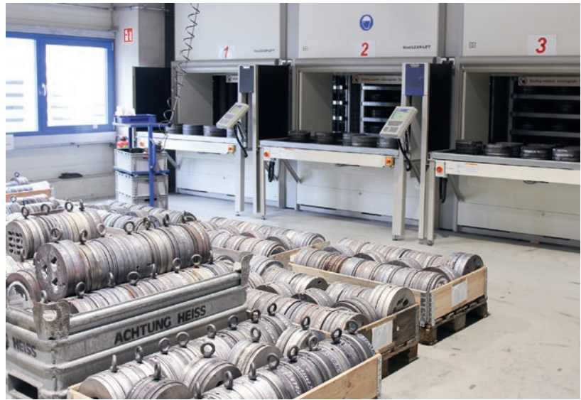
Using different die, the 21-cm diameter aluminium bolts are heated to 470° Celsius and pressed into 50-metre profiles. As a result, each shape has its own tool.
