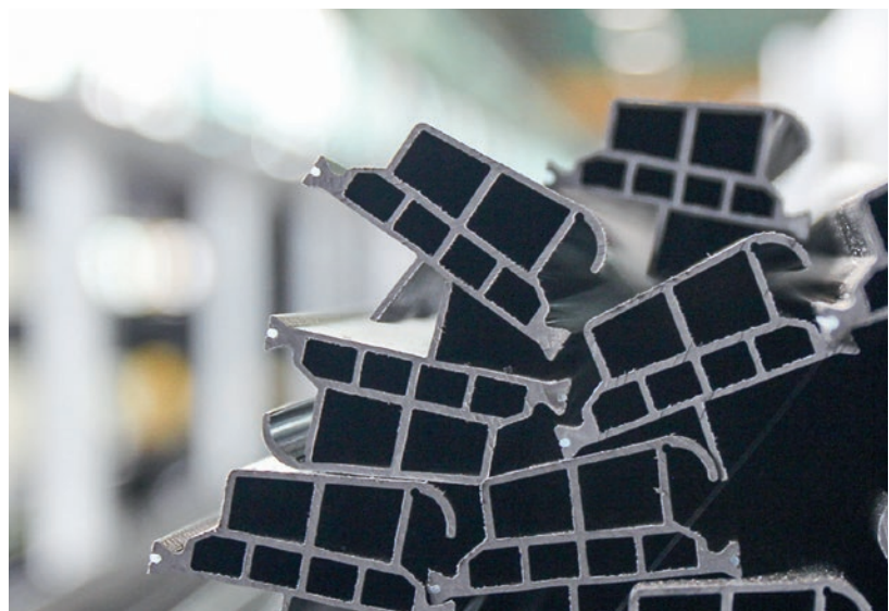
By using polyamide insulation strips, highly efficient composite profiles are produced from the pure aluminium profiles – the polyamide insulation strips and their structure differ depending on the application and requirement.
