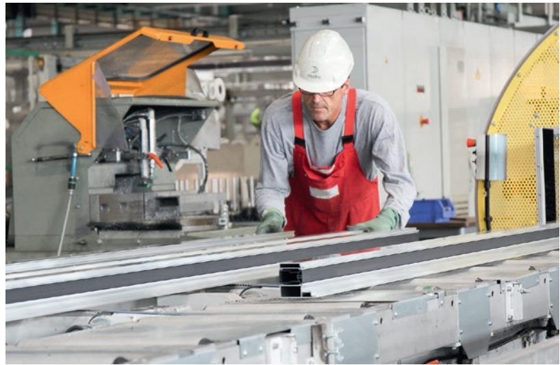
The composite profiles are produced on a total of three machine lines in Bellenberg, where the individual components are assembled manually or by machine.
