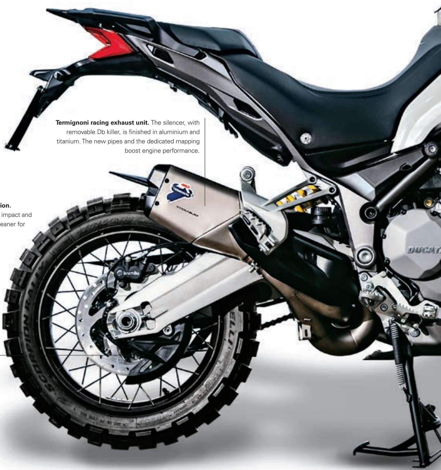
**Termignoni racing exhaust unit.** The silencer, with removable Db killer, is finished in aluminium and titanium. The new pipes and the dedicated mapping boost engine performance.
