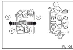
If the turn indicator switch is again operated, while turn indicator is still on, automatic switch-off feature is re-initialised.
