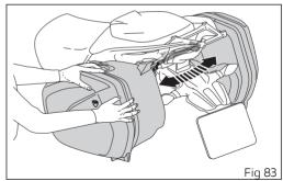
Install both bags, check the swinging movement of both, moving them to the right and left, on the rear side of the bags.
