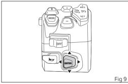
The instrument panel displays the setting screen with the currently set distance selected. Using the joystick ▲ ▼, it is possible to scroll and select one of the 4 distances available. With the same selected distance, the higher the speed of the motorcycle, the greater the distance. The distances indicated are nominal values. Depending on the riding situation and the behaviour of the vehicle ahead, the actual distance may be less or more than these target distances:
