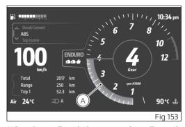
When the needle wake becomes amber yellow and starts blinking, the instrument panel is warning the rider to shift up.
