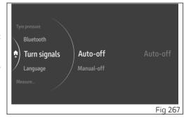
This means that automatic switch-off is triggered when vehicle speed exceeds 20 km/h (12.4 mph) after the turn indicator button was pressed. Turn indicators also switch off automatically if they remained on for a long mileage, which can range between 200 and 2000 metres (656-6562 feet), depending on vehicle speed when the turn indicator button was pressed.
