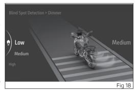
ambient lighting conditions, it may not be possible to notice a marked change in brightness setting. It is recommended to adjust the brightness so that the level 1 information warning does not distract or disturb the view while riding. The brightness of the level 2 hazard warning is linked to the brightness of the level 1 information warning and is automatically adjusted together with it.
