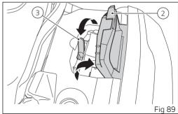
Holding it by the handle (2), pull the side bag (6) out of the housings (5) in hooks (4), first pulling out the rear and then the front, and from the lower support (7).
