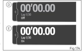
steadily for another 5 seconds, after which it returns to display the time of the current lap, updating the number of laps. When the 30th lap is reached, the message "Full memory" is displayed and it is not possible to record new times: in this case, delete the saved laps in order to record new ones.
