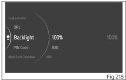
The backlight of the instrument panel is automatically adjusted according to the ambient light detected by photodiode (A, Fig 219). The backlighting intensity adjustment is calculated in relation to what is detected by the photodiode.
