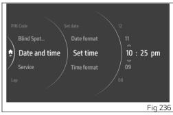
The minute number becomes selectable and is displayed with two arrows placed above and below it; the available values are also displayed (Fig 237). Using the joystick  $\blacktriangle \blacktriangledown$  it is possible to scroll and select the desired value. Press ENTER to confirm and move on to the AM/PM selection.
