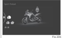
Upon accessing the sub-menu of each profile, levels 1 to 24 are displayed on the left-hand side. While the currently set level is shown on the right. The motorbike is shown in the middle with the part involved in the setting highlighted and the reference indications.
