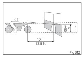
Switch low beam on and cover the right low beam. Adjust the uncovered low beam (left) vertically by working the adjusting screw (1). To reach the screw (1) more easily, it is advisable to turn the steering fully to the right, turn screw 1 with your fingers or, if necessary, with a coin positioned on the notch of the screw (1) to facilitate adjustment if resistance is found.
