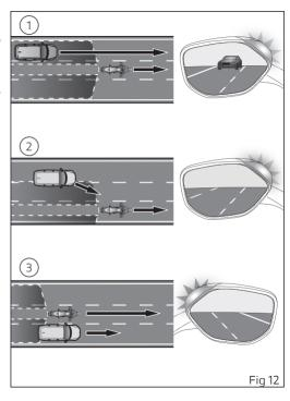
A vehicle that travels in the same direction as the motorcycle, if detected, is signalled by the BSD system even if it enters a blind spot from one side (from the right or left). Like in case 1, this warning can be output earlier if the relative speed of the vehicle with respect to the motorcycle is particularly high.
