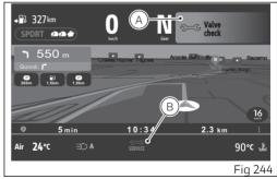
As the thresholds set for service coupons approach, upon each Key-On the instrument panel activates the relevant indications for 5 seconds in large mode (A) in yellow, showing the remaining distance or days: for "Oil service" (C) and "Valve check" (D) it is activated 1,000 km (621 miles) before service is due, for "Annual service" (E) 30 days before service is due.
