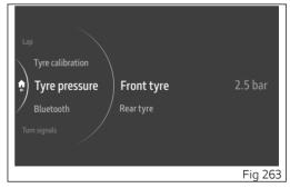
When "Front tyre" (Fig 264) or "Rear tyre" (Fig 265) is selected, the current pressure value is displayed with two arrows at the top and bottom to indicate that the value can be increased or decreased in the relevant joystick ▲ ▼ positions. The currently set pressure is shown on the right. Press ENTER to confirm and return to the previous screen.
