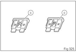
A blown fuse can be identified by breakage of the inner filament (E).
