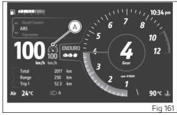
red: the system is in error. Speed control is not active.
