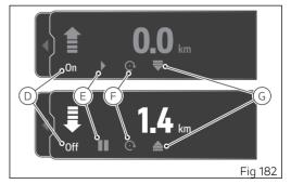
If the meter in differential mode reaches 0.0 km or miles, the Trip master count is paused and the counting mode is changed to incremental.
