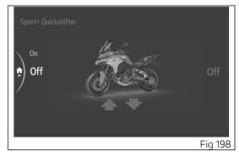
The system works in a separate way for upshifting and downshifting, and combines the action on ignition advance and injection, available in the upshift system and with controlled throttle opening for operation during downshifting. Here below are some tips that will ensure you properly exploit this feature:
