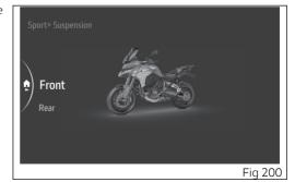
By selecting the items "Front" (Fig 201) or "Rear" (Fig 202), "Hardest", "Hard", "Medium", "Soft", "Softest" levels are displayed on the left-hand side. While the currently set level is shown on the right. The motorbike is shown in the middle with the part involved in the setting highlighted and the reference indications.
