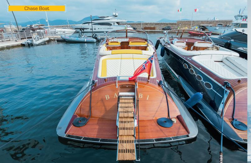
Babebi is a Torpedo «RS» which comes with two Volvo Penta IPS 650s that will take it to a top speed of 47 knots
