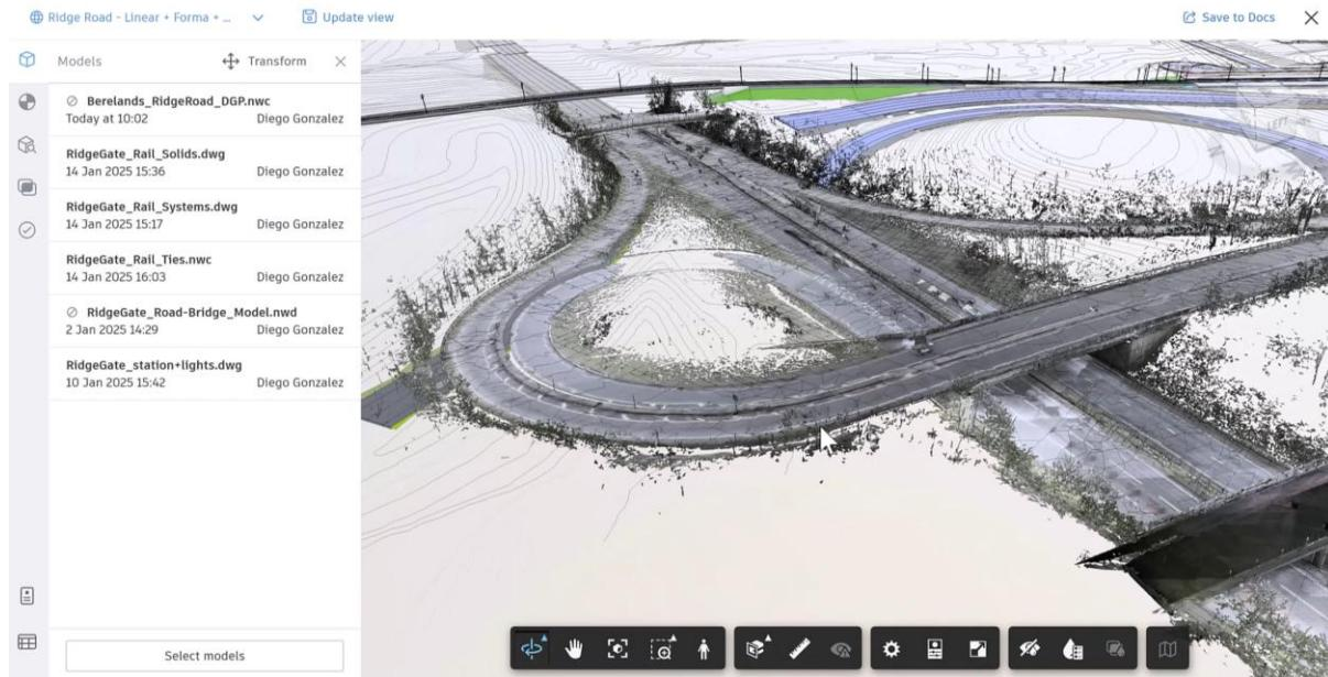
It is worth noting that if the point cloud is classified within **ReCap Pro**, the meshes can be broken down into different sub meshes, this is particularly convenient because this makes possible the independent object creation of meshes, which will potentially be usable within ACC as objects for a proper **clash detection**, an Asset reference within either **ACC Build Assets** or **Autodesk Tandem**.
