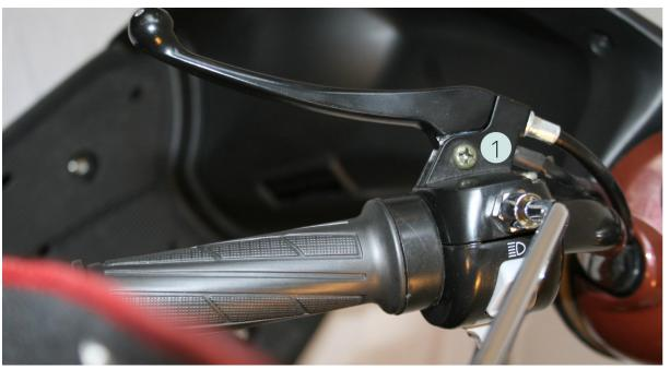
Unscrew the brake cable with the cross-headed screw [1]
