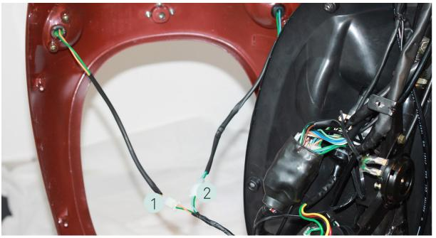
Unscrew the 2 cross-head screws and remove the left-hand indicator from the front plate and unplug it at [1]. Analogue for the right turn signal, unplug the connection at the plug [2].
