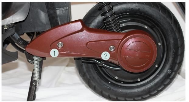
• Unscrew [1] and [2] with a 10mm hex bolt and remove the cover
