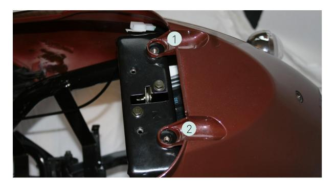
• When assembling, pay attention to any small gap dimensions and position the tabs [1] and [2] carefully above the screw holes.
