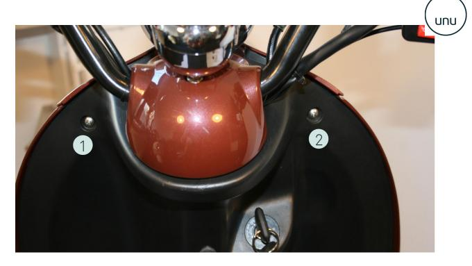
• Unscrew the top cross screws [1] [2] on the front panel back
