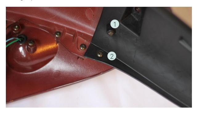
• Unscrew the 4 cross-head screws from the inside. The picture depicts [1] and [2], the other screws can be found on the other side of the number plate rack.
