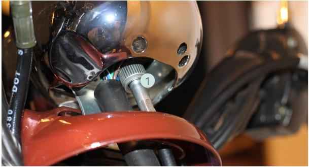
Unscrew the speedometer cable at the connection [1] to the speedometer display. To make sure the nut does not slip too far into the wiring, fix an adhesive strip on the cable 3 or 4 cm under the connection.
