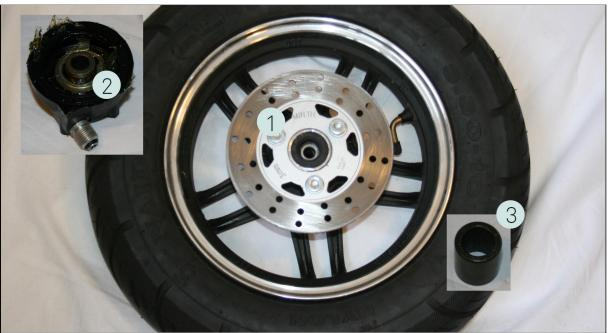
• Fix the opposite side [1] with a 14mm hex bolt and unscrew in opposite directions. Pull the axis out and remove the front wheel. Please beware that the speedometer [2] and spacer bushing [3] are not screwed in and that the brake disk can be threaded out of the brake calipher without great resistance.
