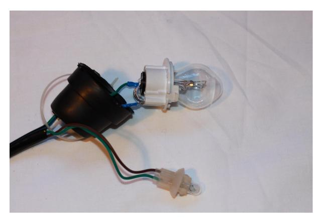
• Info: The parking light bulb is plugged in and it can be pulled out directly to change it.
