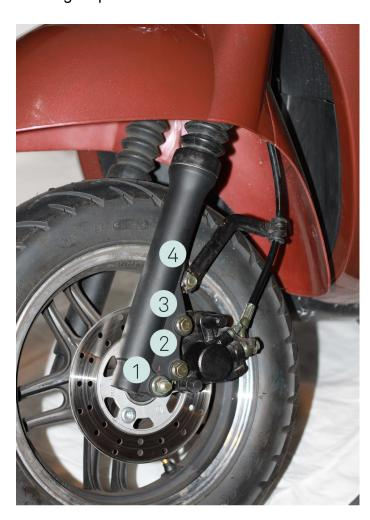
• If the brake caliper isn't removed yet, unscrew the bolts [2] and [3] (12 or 13mm hex bolts) and take the brake caliper from the braking disk.
