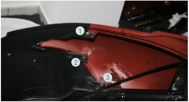
• Unscrew the cross-head screws [1],[2] and [3] on both sides and loosen the interconnected part at each screw by lifting the rear of the joint on the painted panel of the unpainted part.
