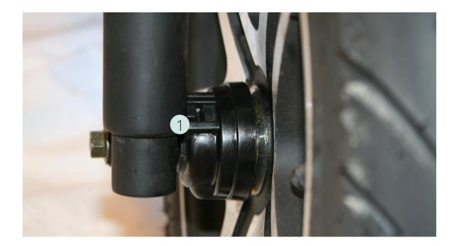
When assembling, make sure that the slot on the speedometer gear is located on the latch on the front fork.
