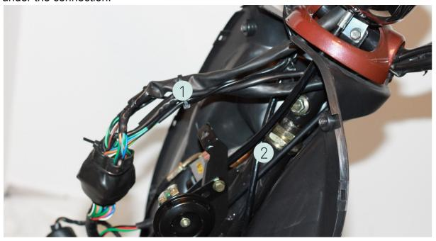
Unplug the speedometer connector from the wiring harness [1].
