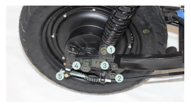
• Unscrew the adjusting nut [5]. This will release the rear brake cable, so you can thread out the cable.
