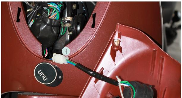
• Disconnect the front light connector [1] from the cable harness
