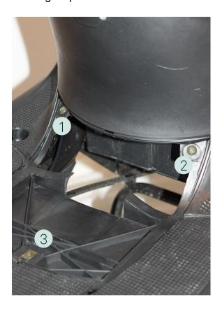
• Unscrew the cross-head screws [1] and [2] under the insert in the footboard
