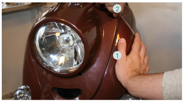
Press one hand for stabilization slightly against the front shield [1]. Use the other hand [2] to
