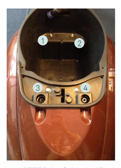
• Unscrew the four screws [1][2][3][4] (10mm Sechskant) and lift the battery container upwards together with the seat. The luggage rack, already dismantled in this picture, can remain on the vehicle for the removal of the battery holder.
