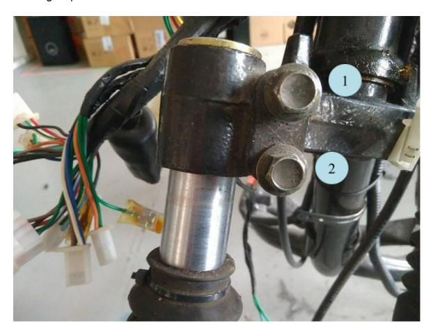
• Unscrew [1] and [2] both 12mm hex bolt on both shock absorbers. Do not remove one screw before the other is loosened as well, unscrew both bolts gradually at the same time.
