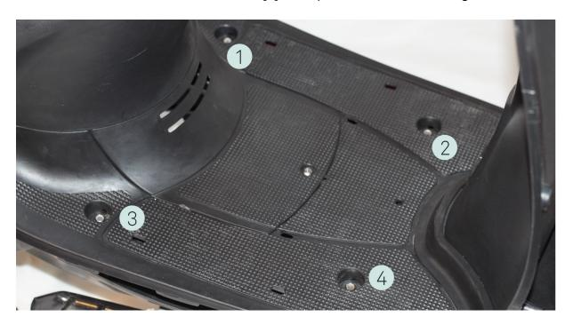
• Unscrew [2] and [4] with a 10mm hex bolt. (Screws [1] and [3] are removed in later parts)
