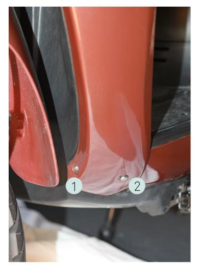
• Unscrew the cross-head screws [1] [2] on both sides, the picture above shows the left side (analogue on the right side)
