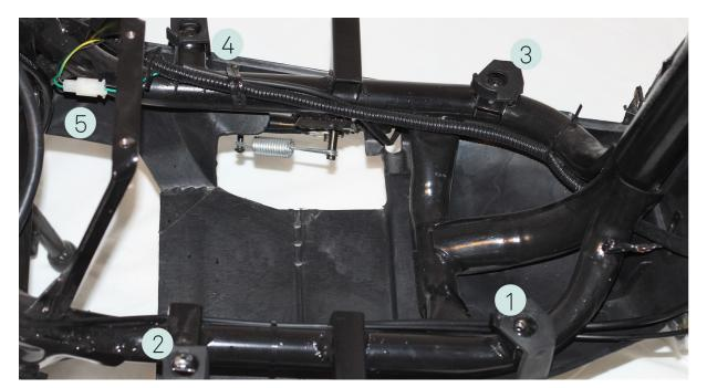
• Press the joint bars of the lower panel [1] [2] [3] [4] to the side and remove the underfloor cover.
