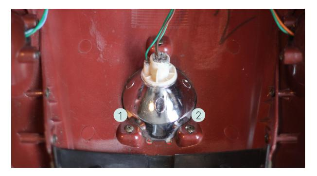
Remove the 2 cross-headed screws [1][2] and take out the backlight.
