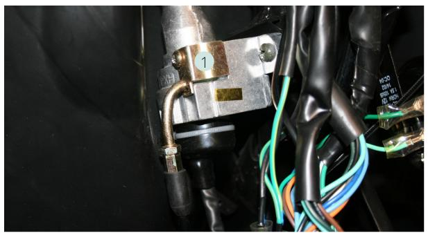
• Unscrew the cross-headed screw screw [1] and unthread the Bowden cable.
