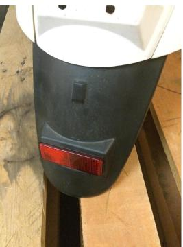
Unscrew the nut (10mm hex bolt) and remove the reflector.
