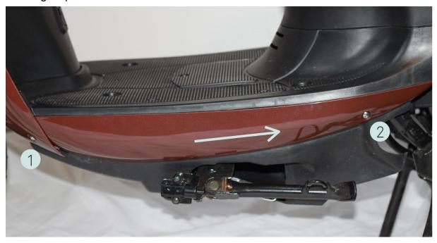
• Unscrew the cross-head screws [1] and [2] and pull the left side panel ca. 2 cm in direction of the rear wheel (see arrow). Afterwards pull the whole panel sideways away from the unu.
