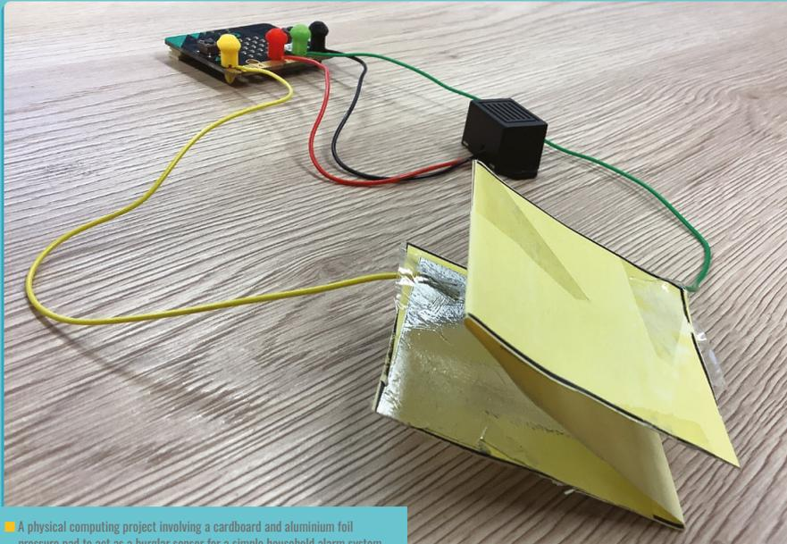
■ A physical computing project involving a cardboard and aluminium foil pressure pad to act as a burglar sensor for a simple household alarm system
