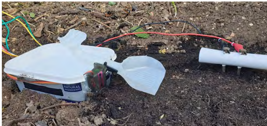
■ Figure 5 The system in situ: reservoir and water pump on the left and soil moisture sensor on the right
