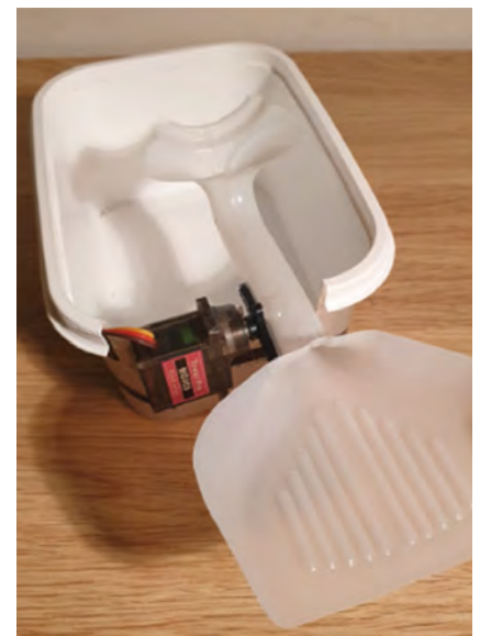
■ Figure 4 A milk carton was cut for the lever scoop
