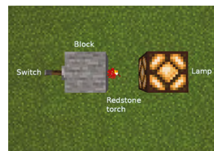
■ Figure 2 A switch is mounted on a block and connected to a lamp via a redstone torch: when the switch is off, the lamp is on, and vice versa
