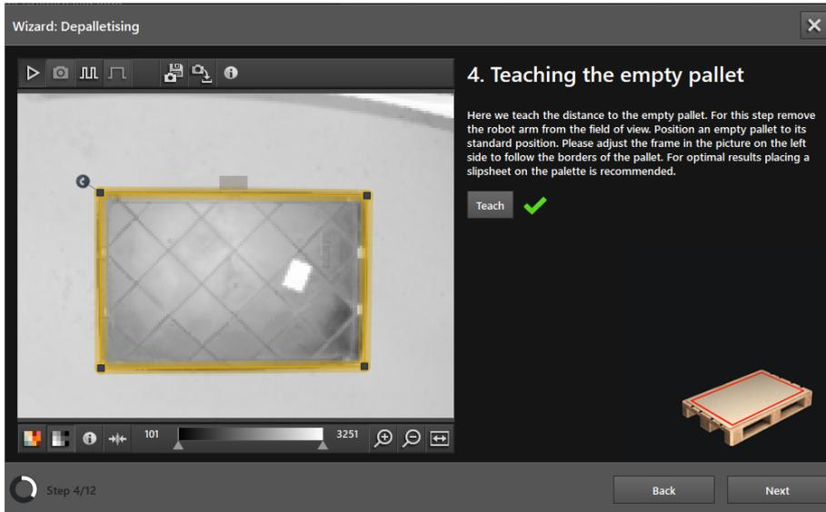
The reference level is taught in the "Teaching the empty pallet" window. The surface of the empty pallet is defined to be the reference plane.
