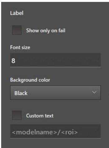
The checkbox [Show only on fail] links labelling of the ROIs with their state. If the checkbox is activated, labelling of the ROIs is only shown if the state is "failed".
