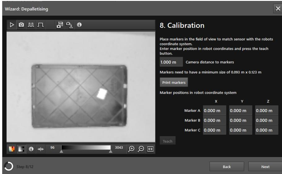
The coordinate system of the device is combined with the coordinate system of the robot in the "Calibration" window.
