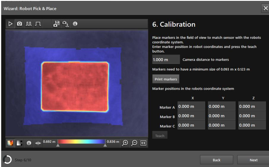
The coordinate system of the device is combined with the coordinate system of the robot in the "Calibration" window.
