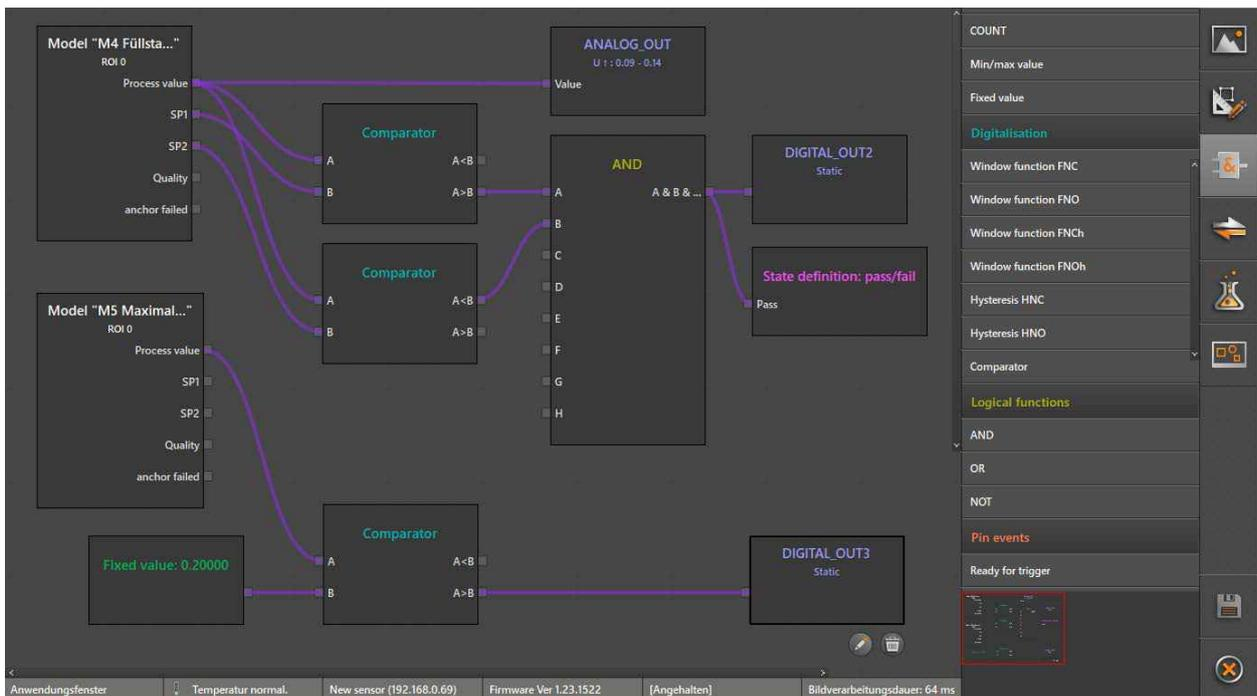
> This logic is used to verify if the process value is greater than the fixed value. If this condition applies, the digital output is switched.
