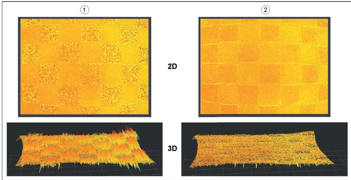
1: An exposure time of 500  $\mu$ s, white surfaces almost saturated, black surfaces noisy
