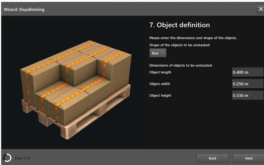
The dimensions and shapes of the objects are set in the "Object definition" window.
