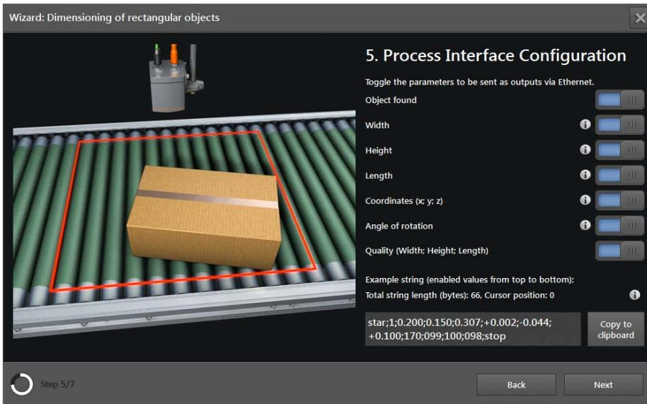
► Select via the buttons which parameters are to be transmitted via the process interface (Ethernet).
