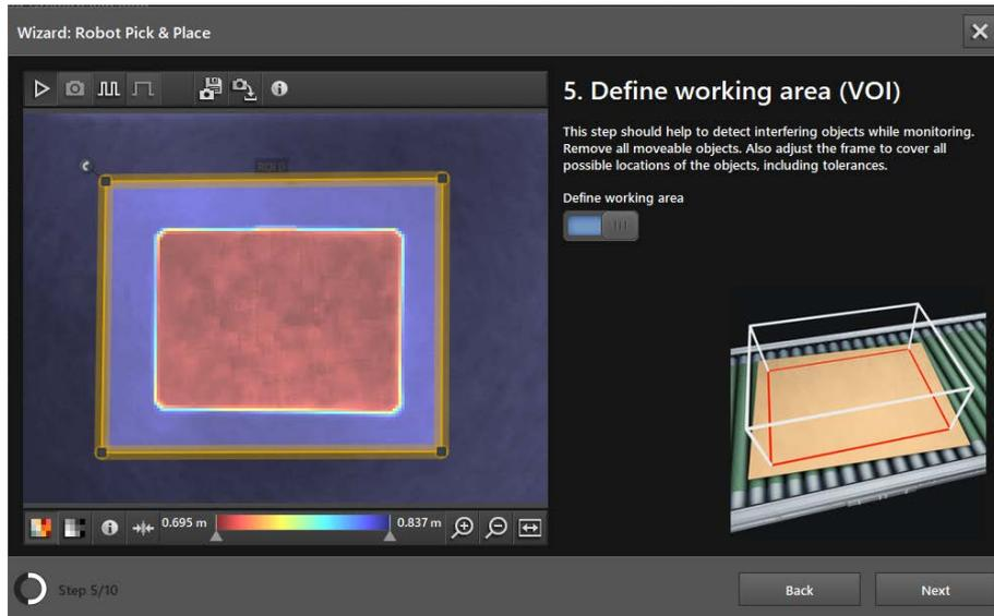
The working area is set in the "Define working area (VOI)" window. The working area defines the area in which the object is to be detected.
