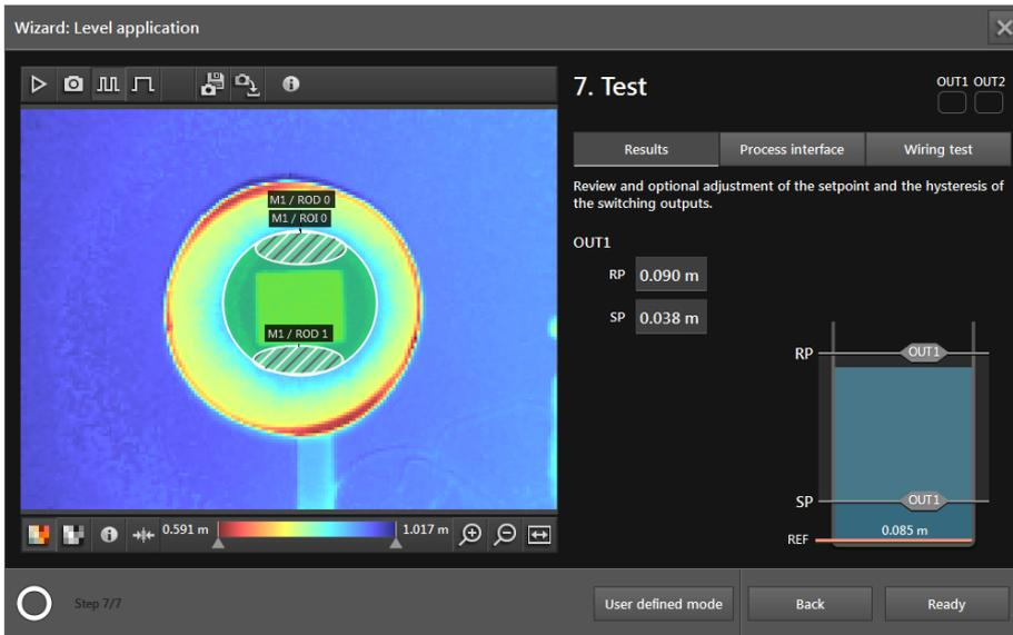
In the final step the functions of the application are tested:
