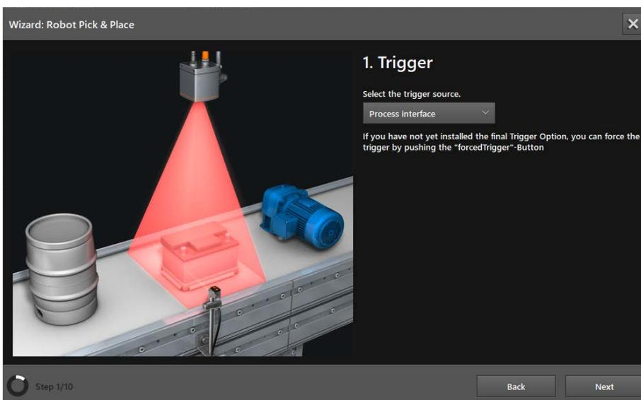
The trigger for the image capture is set in the "Trigger" window.
