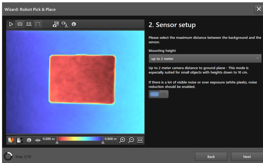
The distance between the device and the background (reference plane) of the objects are set in the "Sensor setup" window.
