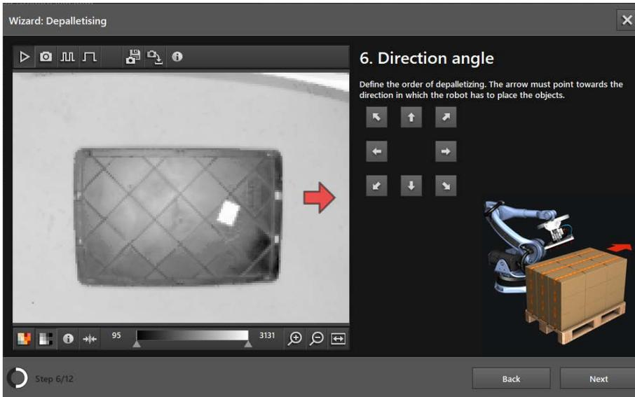
The direction in which the robot unstacks the objects (depalletising direction) is defined in the "Direction angle" window.
