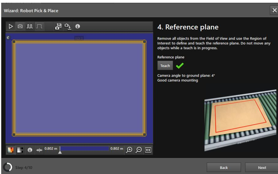
The reference plane is taught in the "Reference plane" window. The base plate of the objects is defined to be the reference plane (e.g. conveyor belt).
