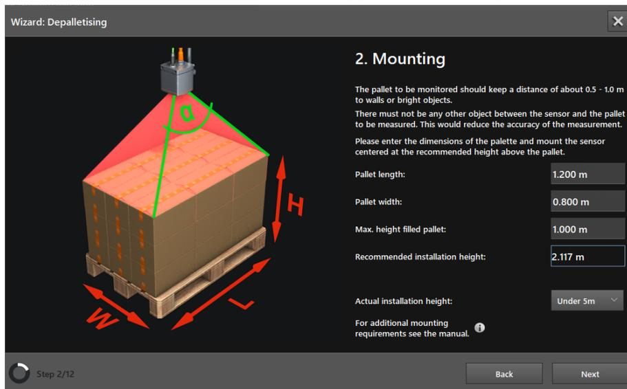
The optimum installation height of the device is recommended in the "Mounting" window.
