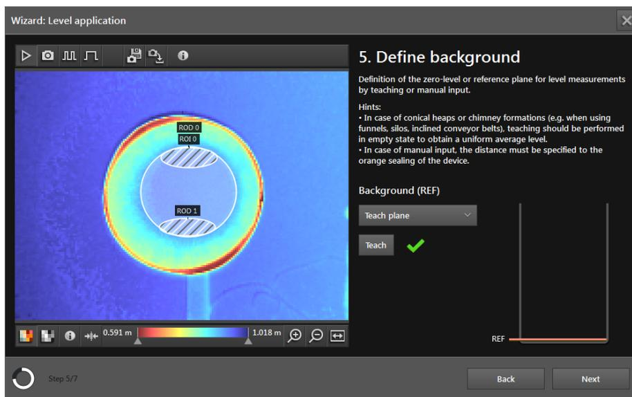
The window "Define background" determines the reference or zero plane of the level measurement. It can either be set (use an average value from 20 measurements on an empty container) or entered manually.
