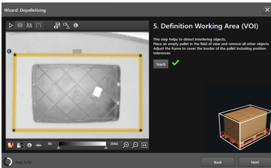
The working area is set in the "Definition Working area (VOI)" window. The working area defines the area in which the pallet is to be detected.
