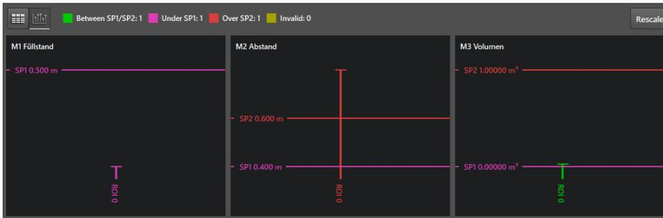
The process values of the individual ROIs are indicated as vertical lines in the bar graph. The line colour shows the status of the ROIs. The switching thresholds are represented by horizontal lines.
