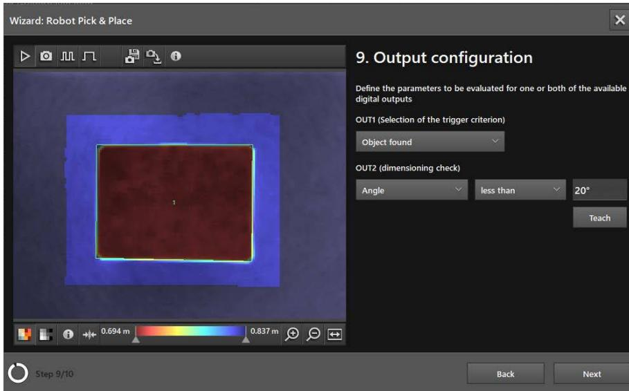
The output is set via the digital outputs in the "Output configuration" window.
