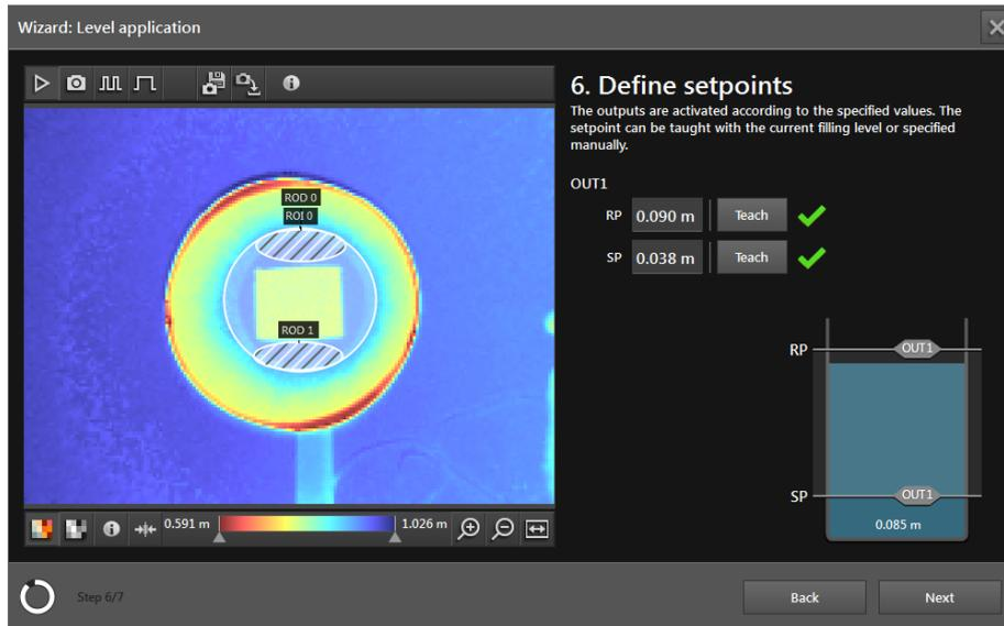
The outputs are switched according to the definition of the setpoints. Each setpoint can either be entered manually or set with an appropriate quantity of the product in the container.
