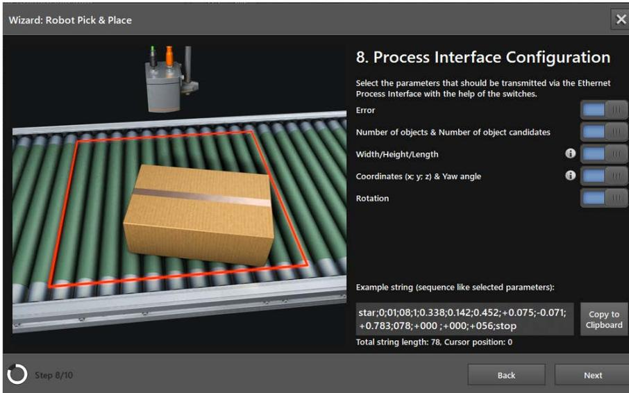
The output is set via the process interface in the "Process Interface Configuration" window.
