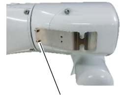
Hexagon socket head cap bolt 2-M4×10
