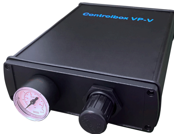
Figure 7: Front panel of the SoftGripping Control Box.
