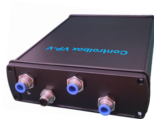
Figure 6: Back panel of the SoftGripping Control Box.
