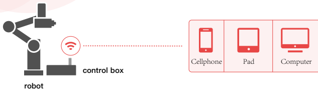
Figure 2.3 Wireless network connection topology diagram
