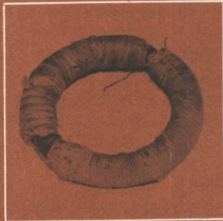
The original iron ring used by Faraday in this experiment. Royal Institution
