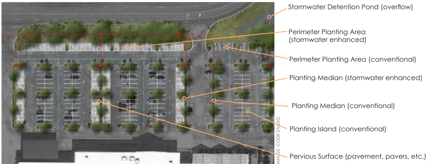
CH7-44: An illustrative example of how the parking lot might be transformed with the application of integrated landscaping and stormwater management approaches. The example above mixes both conventional and stormwater enhanced approaches.
