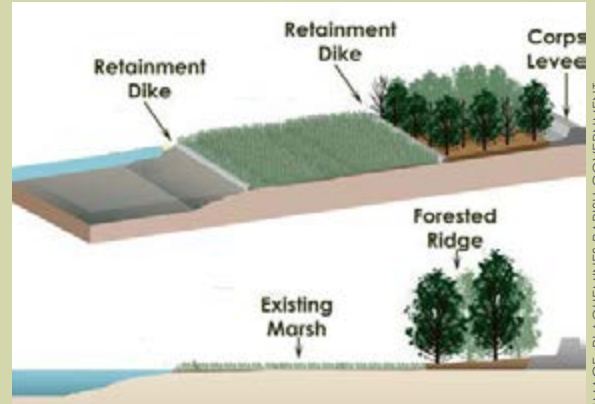
CH5-17: Forested ridge improvements result in the reduction of the wave action on top of tidal surge to a level below levee height.
