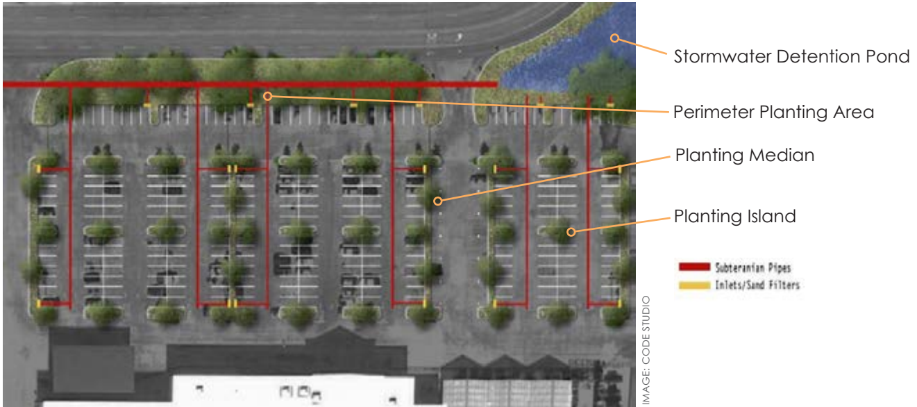
CH7-43: An illustrative example of how the parking lot might be transformed with the application of conventional landscaping and stormwater management approaches.
