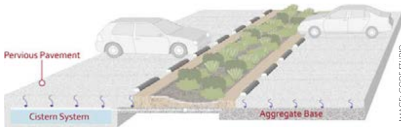
CH7-51: An illustrative example of a stormwater enhanced planting median area as outlined by the Coastal Toolkit. This example shows two optional stormwater management devices where pervious pavement or pavers are placed on top of an aggregate fill or cistern storage system.
