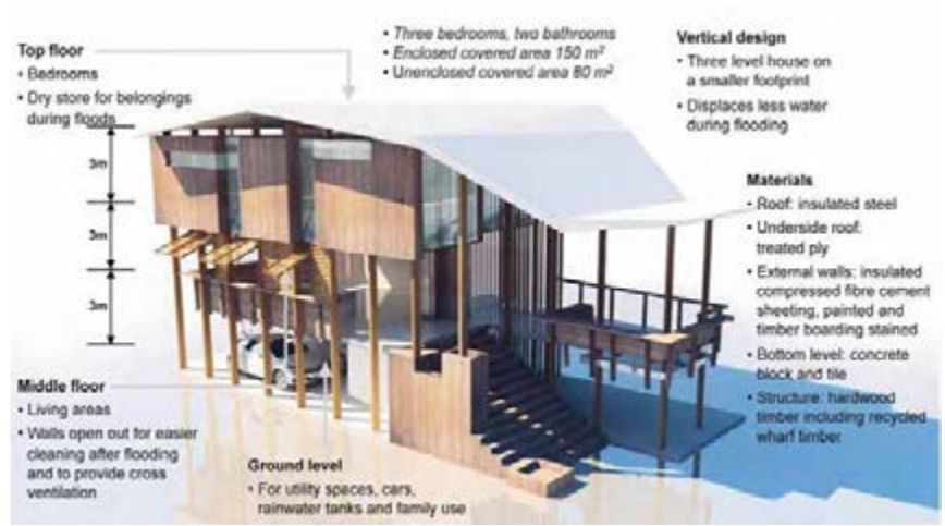
CH2-19: The “Queenslander House” is a model home that is flood resistant. The Government promotes this type of design for those living in at risk areas.
