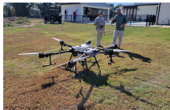
Large drones used for spraying crops are now being used to spray ripening agents on sugarcane, a job once reserved for crop dusters and helicopters. (Photo by Randy Price)
