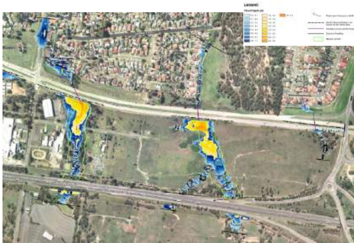
Figure 4.1. Hyder Flood Study – 1% AEP Flood Extent – Pre-development
