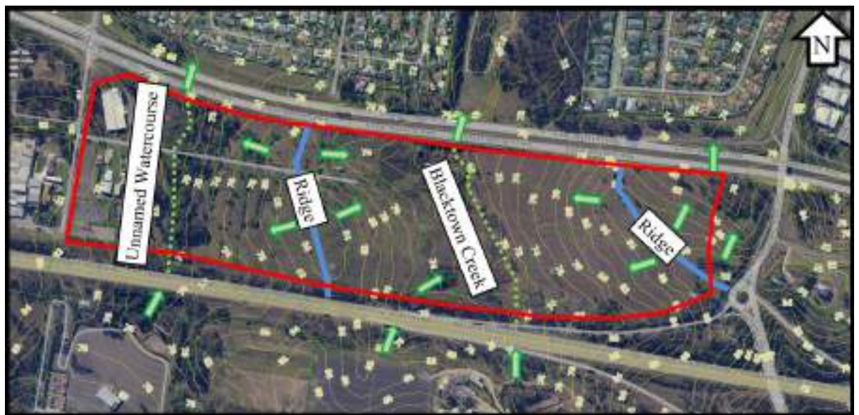
Figure 2.3. Site General overland flow drainage (Source: Nearmap 16 June 2022)
