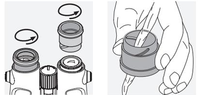
In the event of hard-to-remove dirt (e.g. sand) the eye cups can be unscrewed and cleaned easily.
