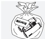
If the instrument is wet, it must be dried prior to storage.
