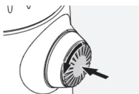
Press on the knob and rotate it counterclockwise (90°).
