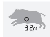
Moving targets are measured continuously in scan mode. The instrument automatically switches to scan mode if you press and hold the measurement button for longer than 3 seconds.
