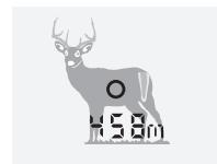
Briefly press the measurement button to display the target mark. After releasing the button, the range measurement is shown in the display.
