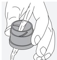
**Cleaning the protective housing.** Use the soap & brush kit (supplied). Close the covers on the eyepiece and objective lenses. Remove the battery and close the battery compartment before cleaning. Moisten the brush and apply the soap using circular movements to gently clean the housing. Then rinse the device with clean water and dry it with care. If the optics become wet, dab them dry with a clean cloth to prevent scratching. Rinse the brush thoroughly and leave the soap & brush kit to dry.
