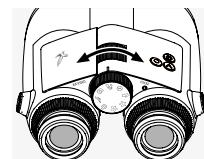
Turning the focusing wheel allows you to focus on any object from the shortest focusing distance (see technical data sheet) to infinity.
