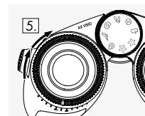
4. Use the focusing wheel to focus the right channel on a distant object (keep the left eye closed).
