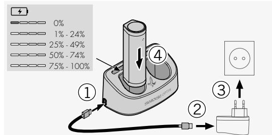
The AX VISIO is supplied with the RB battery installed. Please charge the battery fully before using the device for the first time (see 4.2).
