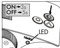
**SWITCHING ON:** Press and hold the ON/OFF button for at least three seconds until the LED status indicator changes from yellow to green. The AX VISIO is now switched on and is starting up. The LED status indicator flashes for around 30 seconds. After this, the LED status indicator turns permanently green. The AX VISIO is now ready to use and the display is active.
