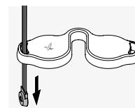
If you want to fit an eyepiece cover or other accessory, pull the strap through the eyelet of the cover.
