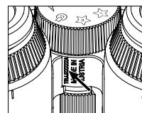
You can find the serial number of your product on the bottom of the device between the mode selection wheel and the focusing wheel. To see the serial number clearly, open the device out fully.
