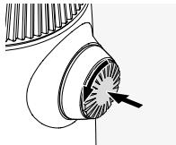
Press on the knob and rotate it counterclockwise (90°).
