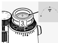
3. Now look through the right eyepiece with your right eye and turn the diopter adjustment ring clockwise until the display is sharp. Then completely remove the objective lens cover.
