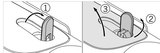
To insert the battery in the device, you first need to open the battery compartment. This is located on the bottom of the device. To open the battery compartment, flip the bayonet closure up to a vertical position (1), turn it 90° counterclockwise to the left (2), and open the battery compartment cover (3).
