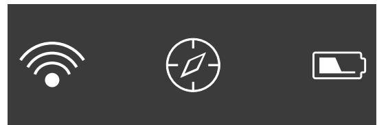
The status bar shows information about the current status of the AX VISIO. On the left, you can see whether there is currently an active Bluetooth or Wi-Fi connection with a smartphone. In the middle, the app currently selected on the mode selection wheel is shown. On the right, you can see the current battery status. The status bar disappears automatically five seconds after starting up the AX VISIO, changing the app on the mode selection wheel, or reactivating the display.
