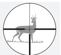
Even at high magnification, only a thin area of the target is covered. The reticle can only be used for estimating the distance to a limited extent.
