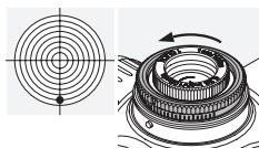
Turn the outer knurled ring on the top turret in the direction of H (counter-clockwise).
