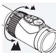
Turn the magnification adjustment ring through up to  $180^\circ$  to obtain the required magnification. The adjustment is continuous. The scale on the adjustment ring makes it easy to see the setting. The soft ribbed cover of the adjustment ring has a small protrusion to make orientation easier.
