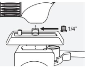
The ATC/STC has a  $\frac{3}{8}$ " UNC connection thread. The bush that has been inserted reduces the thread to  $\frac{1}{4}$ " UNC. The thread can therefore be used to mount an adapter plate and the spotting scope is compatible with all common tripod heads.
