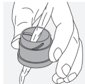
To ensure the long-lasting optical brilliance of your spotting scope, you should keep the glass surfaces free from dirt, oil, and grease. To clean the optics, first brush off any larger particles of dirt using an optical lens brush. Then breathe gently on the lens and polish it with the cleaning cloth to remove any remaining dirt.
