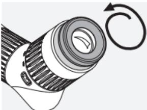
For use without glasses: unscrew the twist-in eyecup (counter-clockwise) as far as it will go.
