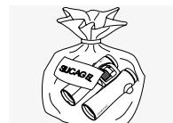
Keep your binoculars in their bag in a well-ventilated place. If the binoculars are wet, they must be dried first. In tropical areas or areas with high humidity, it is best to store them in an airtight container with a moisture-absorbing agent (e.g. silica gel).
