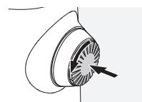
Press on the knob and rotate it counterclockwise (90°).
