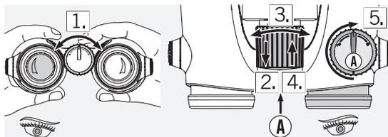
1. Look through the left ocular with your left eye and turn the focusing wheel to focus sharply on a selected object.
