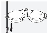
If you want to fit an eyepiece cover or other accessory, pull the strap through the eyelet of the cover.
