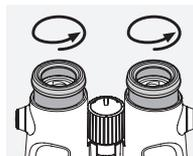
Pos. A: Initial position without spectacles: Twist out the eyecups anti-clockwise to the full extent.
