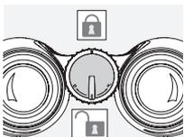
The dioptric lock is secured by turning it 180° in a clockwise direction. Turning it 180° in a counterclockwise direction releases it again.
