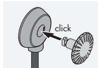
Align the button pin with the strap connector ring and press until it clicks.
