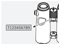
You will find the serial number of your EL binoculars underneath the focusing wheel. In order to be able to read it, the focusing wheel must be pulled out.
