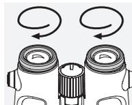
Pos. B: Initial position with spectacles: Twist in the eyecups clockwise until they stop.
