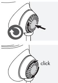
Press the pin in firmly and turn slightly clockwise.
