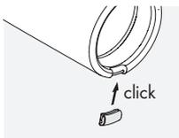
3. Push the protective gap cover provided onto the metal ring. The gap cover is not firmly attached until a click can be heard.
