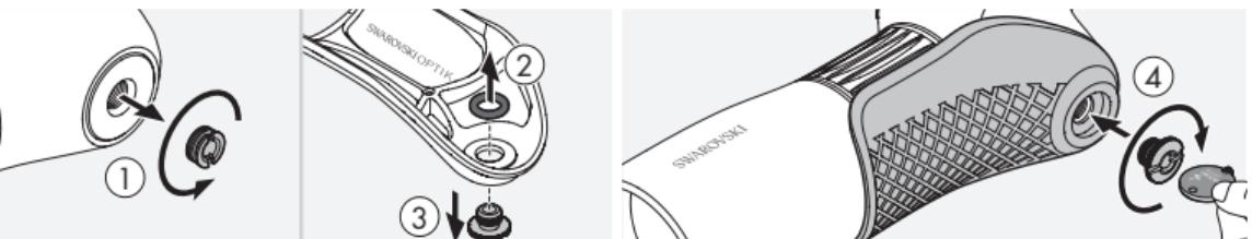
Step 3: Secure the half shell to the bottom of the spotting scope using the locking screw.
