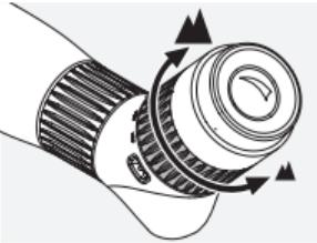
Changing magnification: turning the adjustment ring to the right increases the magnification, turning it to the left reduces the magnification. The index mark shows the current magnification setting.
