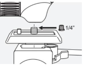
The ATC/STC has a  $\frac{3}{8}$ " UNC connection thread. The bush that has been inserted reduces the thread to  $\frac{1}{4}$ " UNC. The thread can therefore be used to mount an adapter plate and the spotting scope is compatible with all common tripod heads.
