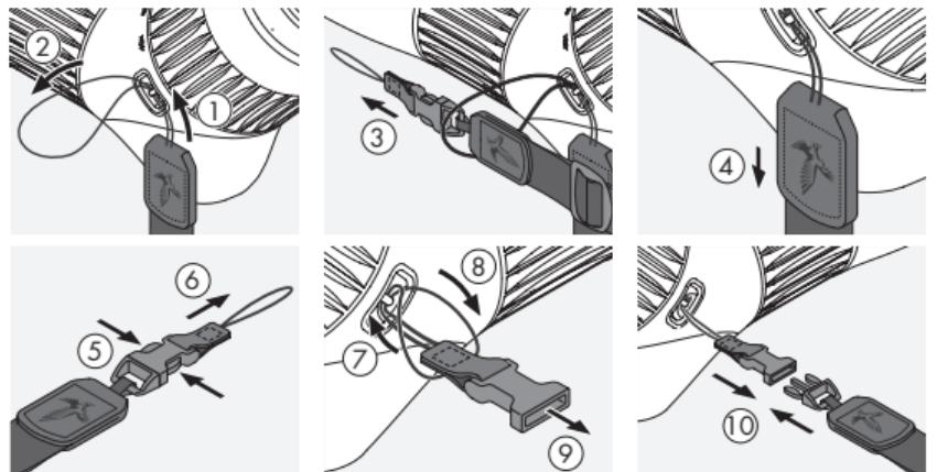
On the other side, release the end of the clip mechanism (5+6) and feed the loop through the loop holder (7). Then pull the end through the loop (8), tighten it (9), and attach the clip to the other end of the side carrying strap (10).
