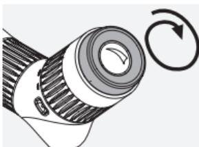
For use with glasses: screw in the twist-in eyecup (clockwise) as far as it will go.
