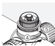
Open the locking mechanism on the marking ring. Turn the marking on the turret to zero if it has moved to another position.
