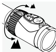
Turn the magnification adjustment ring through up to 180° to obtain the required magnification. The adjustment is continuous. The scale on the adjustment ring makes it easy to see the setting. The soft ribbed cover of the adjustment ring has a small protrusion to make orientation easier.
