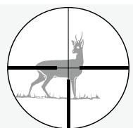
Even at high magnification, only a thin area of the target is covered. The reticle can only be used for estimating the distance to a limited extent.
