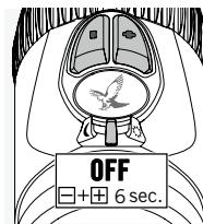
You can deactivate the SWAROLIGHT function by turning the OFF/DAY/NIGHT switch to the central position and pressing the +/- buttons at the same time for 6 seconds. The light will flash twice to confirm that the function is deactivated. You can reactivate the SWAROLIGHT by repeating this step.
