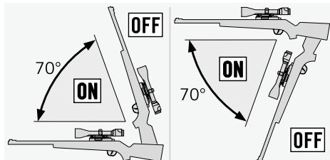
The scope also switches off if the lateral tilt is greater than 30° (if you rest the rifle on your legs, for example).
