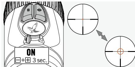
Turn the OFF/DAY/NIGHT switch to the DAY or NIGHT position to switch on the illuminated ring of the FLEXCHANGE 4A1F reticle. The reticle illumination is now activated. Press the +/- buttons at the same time for 3 seconds to switch on the illuminated ring. Repeat this step to switch the ring off again.
