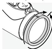
First, turn the diopter adjustment ring fully to the left (counter-clockwise) and then to the right until the reticle is in sharp focus. The adjustment range depends on the individual model.
