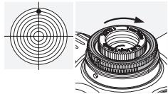
Turn the outer knurled ring on the top turret in the opposite direction to H (clockwise).
