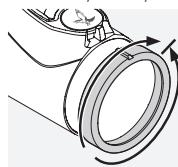
First, turn the diopter adjustment ring fully to the left (counter-clockwise) and then to the right until the reticle is in sharp focus. The adjustment range depends on the individual model.
