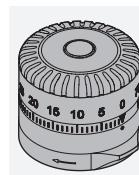
The ballistic turret flex (BTF) can be configured separately and enables you to stay on target at the required distances. If it is used as a top turret, it can compensate for bullet drop. When used as a side turret, it is ideal for windage adjustment or for estimating the lead distance. The BTF can be fitted without tools and can be combined with any available reticle.
