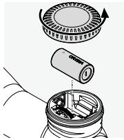
please make sure that the side marked "+" is in the correct position (see marking on the instrument).
