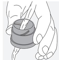
**Cleaning the protective housing.** Use the soap & brush kit (supplied). Close the covers on the eyepiece and objective lenses. Moisten the brush and apply the soap using circular movements to gently clean the housing. Rinse the binoculars with clean water and dry with care. If the optics become wet, dab them dry with a clean cloth to prevent scratching. Rinse the brush thoroughly and leave the soap & brush kit to dry.
