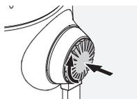
Push the knob in firmly and rotate slightly clockwise.
