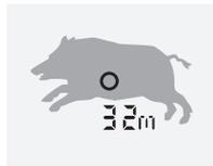
Moving targets are measured continuously in scan mode. The instrument automatically switches to scan mode if you press and hold the measurement button for longer than 3 seconds.
