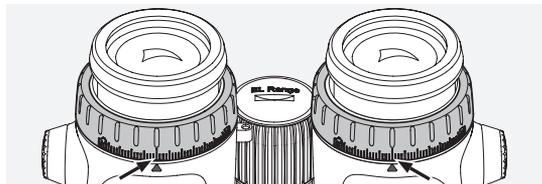
**b.** Then push the diopter adjustment ring back in. If the vision in one or both eyes is impaired, adjust the binoculars as described in 3.4. The display has to be in sharp focus to achieve the best possible performance in determining range.
