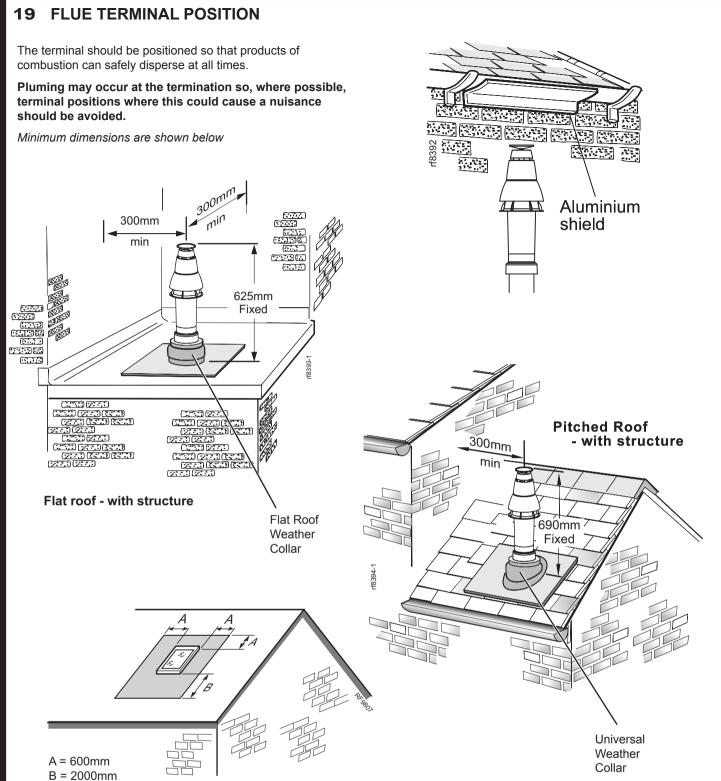
The flue terminal shall not penetrate the shaded area of the roof
