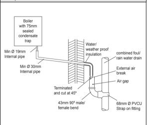
Figure 6 - Connection of Condensate Drainage Pipe Upstream of a Sink, Basin, Bath or Shower Waste Trap to External Drain, Gulley or Ranwater Hopper Boiler with 75mm sealed condensate Visible air break trap at plug hole weather proof Min Ø 19mm insulation Internal pipe Sink, basin, bath or Minimum 30mm shower with integral 2 internal pipe overflow and 75mm trap 45° pipe termination
