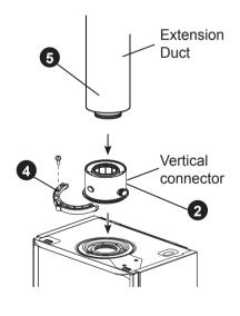
**6.** If the last extension duct requires cutting, measure 'X', the distance (outer ducts), between the duct and the terminal and add 100 mm to this dimension. This gives the length of the last extension duct.
