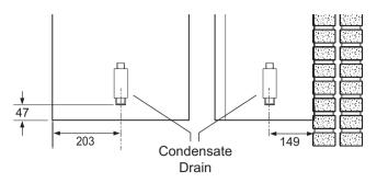
This appliance is fitted with a siphonic 75mm condensate trap system that requires filling before operating the appliance for the 1st time or after maintenance.
