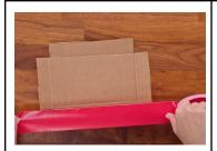
Step 11: Lay the cardboard down and begin covering the boat completely in duct tape, front and back. It helps to cover one side at a time with strips that reach the length of the cardboard. Wrap any overhanging tape around the sides of the cardboard.
