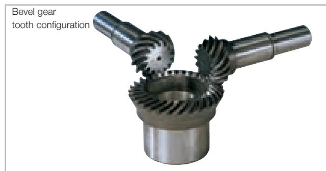
The tooth profile play (when new) of 0,1 – 0,3 mm varies, depending on the size of the unit resp. centre distance of shaft to wheel, with the rate of wear.
