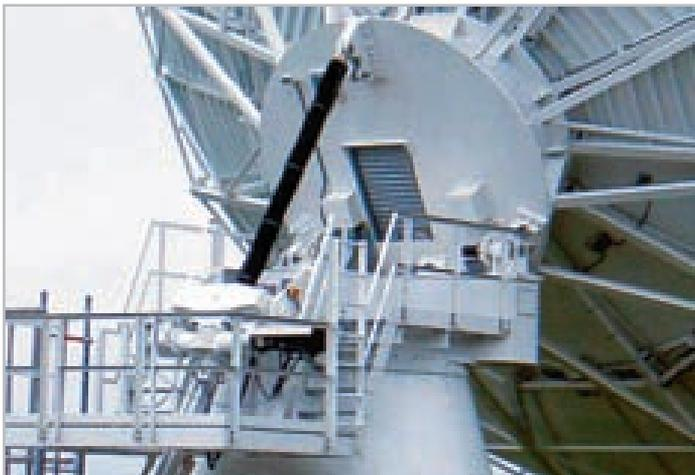
HSE high performance worm gear screw jack, special configuration for an elevation movement from 0 °C to 90 °C of an 11,1 m antenna.
