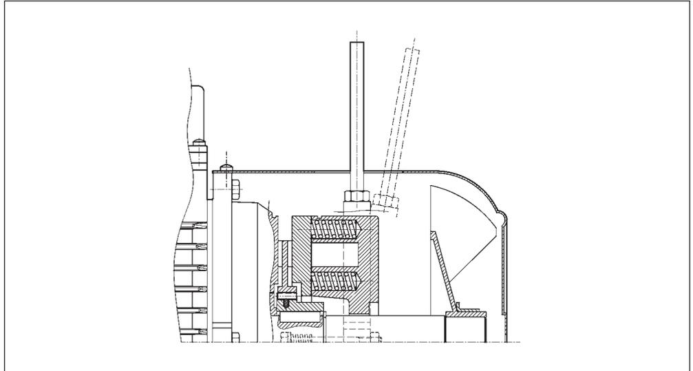
On motors type BN\_FD, if the option RM is specified, the release device may be locked in the "release" position by tightening the lever until its end becomes engaged with a brake housing projection. The availability for the various disengagement devices is charted here below:
