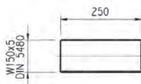
Material: Case hardening steel 18NiCrMo5 UNI 5331 must be case hardened 50-55 HRC
