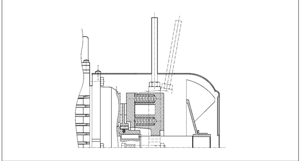
A return spring brings the release lever back in the original position.
