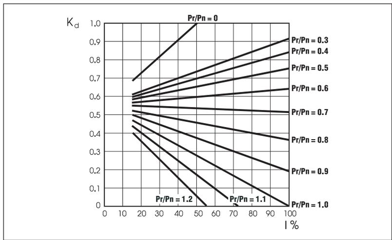
If actual starts per hour is within permitted value ( $Z$ ) it may be worth checking that braking work is compatible with brake (thermal) capacity  $W_{max}$  also given in tables (F30), (F38) and dependent on the number of switches (c/h).
