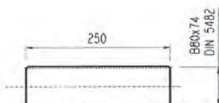
Material: Case hardening steel 18NiCrMo5 UNI 5331 must be case hardened 50-55 HRC
