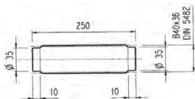
Material: Case hardening steel 18NiCrMo5 UNI 5331 must be case hardened 50-55 HRC
