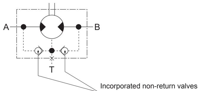
1) If the drain port is connected up, pressure at the shaft seal is always equal to the pressure in the drain line.
