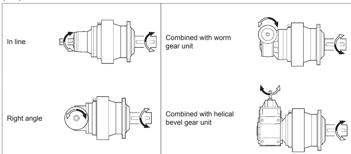
**RA/RO:** For the monodirectional applications or for the applications requiring a sense of rotation prevailing on that opposite to it, the selection of "**RA/RO**" option ensures the declared performance. For applications not requiring a prevailing sense of rotation with respect to each other, the performances are guaranteed regardless of the selected "**RA/RO**" option.
