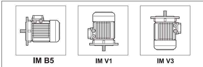
Flange output motors are also available with reduced coupling dimensions, as indicated in the table below - executions **B5R**. Their use in combination with gearboxes must be however coherent with the maximum installable power on gearboxes themselves (see chapters "Motors availability"). In case this condition is not met need to contact the Technical Service for the checking of the combination.
