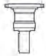
**VK:** Reinforced output with heavy duty keyed shaft for stirrers and mixer
