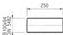
Material: Case hardening steel 18NiCrMo5 UNI 5331 must be case hardened 50-55 HRC
