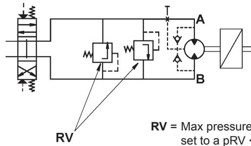
**RV** = Max pressure secondary valve set to a  $p_{RV} < p_{max}$
