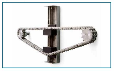
The double-tensioner for chain drives with reverse operation. Thanks to the "floating" suspension of the clamping elements, the tension is always applied just where it's needed: On the slack strand.
