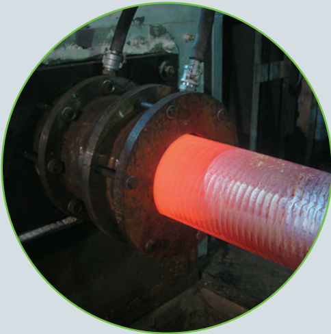
THE PROCESS OF CASTING BRONZE TUBES
