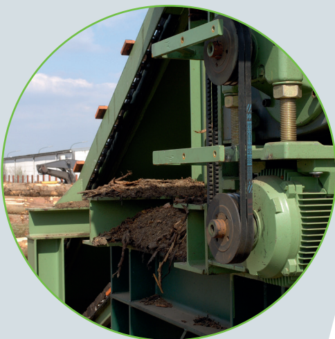
V BELT DRIVES FOR SAWMILL MACHINERY
