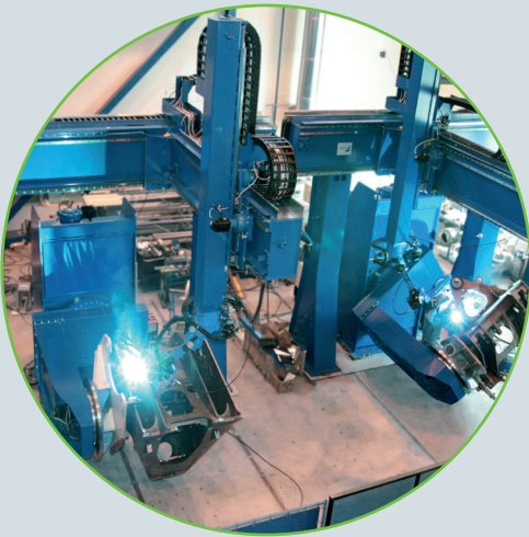
ROBOT WELDING STATION
