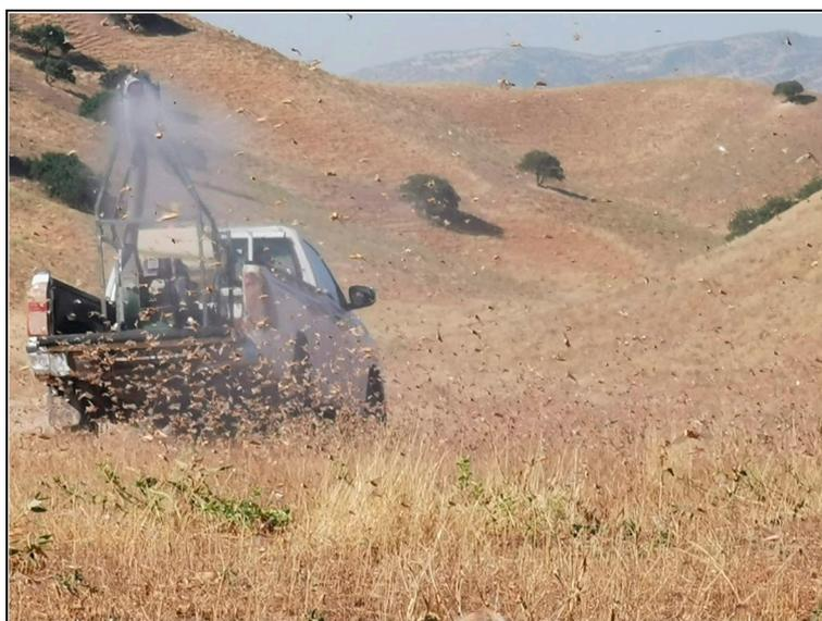
**Figure 15.** Treating a swarm of adult Moroccan locusts with the vehicle-mounted ULV sprayer Micron AU-8115. Photo: Oleg T. Guchgeldyev.
