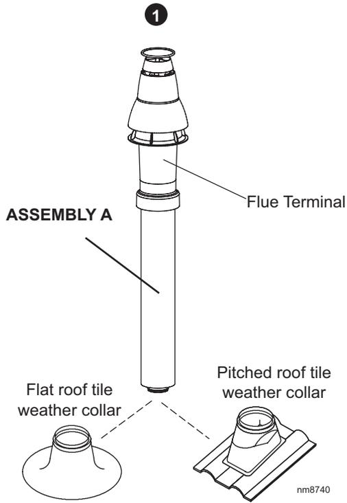
2. Fit the vertical connector (supplied in kit) in accordance with the instructions provided with the vertical connector kit.
