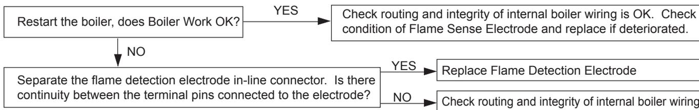
**RESTART PROCEDURE** - To restart boiler, press and release RH push button.
