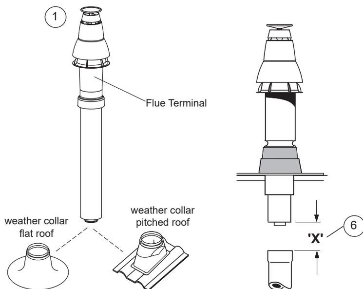
5. Push extension duct (if required (supplied separately)) into vertical connector.
