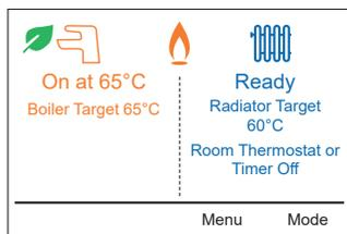
2. Close all taps except the furthest one from the boiler and check that the boiler is firing at maximum rate. This is factory set to give a DHW temperature rise of approximately 35°C at the flow rate stated on page 8 under "operation".
