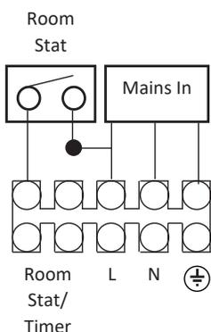
**Diagram D: OpenTherm Programmable Room Stat**
