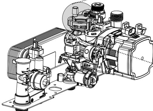
5. Reassemble. Ensure the air vent head 'o' ring seal is fitted.
