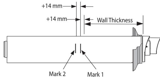
7. Place the terminal end of the flue into the 127 mm core drilled centrally and slowly apply slight pressure and move the flue up or down or side to side. This will cause the external wall seal to fold in and allow the flue to pass through the wall.
