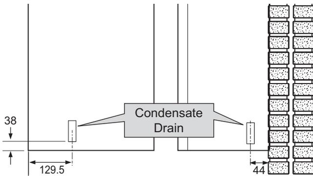
This appliance is fitted with a siphonic 75 mm condensate trap system that requires filling before operating the appliance for the 1st time or after maintenance.
