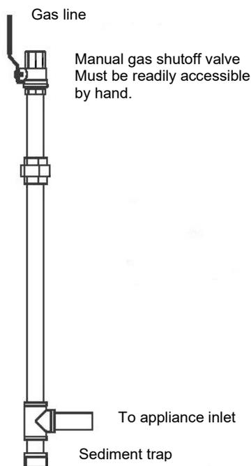
Install a manual "Equipment Shut-Off Valve". This valve is part of the boiler / water heater delivery. Should overheating occur or the gas supply fail to shut off, turn off the manual gas control valve. The gas line piping can safely be removed from the appliance for servicing. Leak test the gas pipe from the boiler / water heater up to the gas pressure regulator. Carefully vent the gas pipe (outside in open air) before putting the appliance into operation for the first time;
