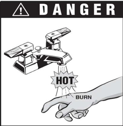
Water temperature over 125°F can cause instant severe burns or death from scalds.
