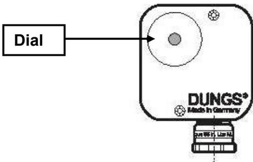
1. Remove the cover from the gas pressure switch
