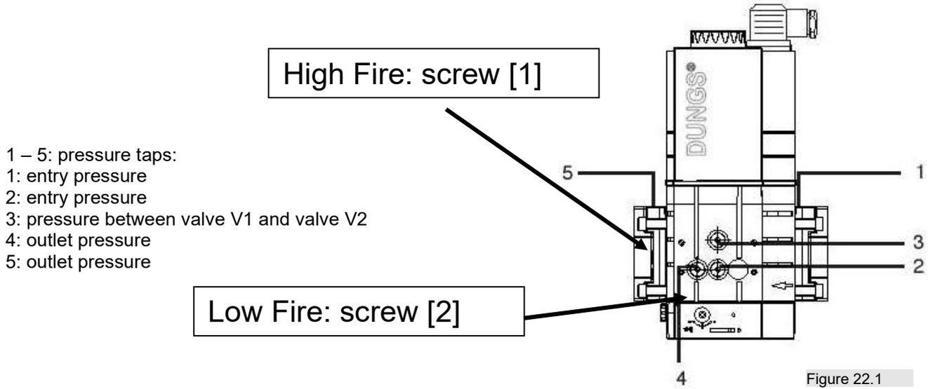
**High Fire:** adjustment screw: use small flat screwdriver
