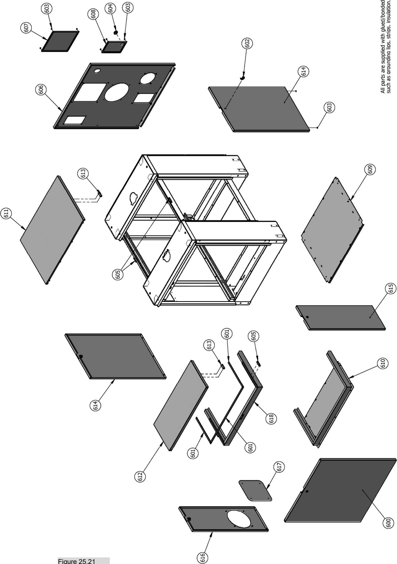
All parts are supplied with glued/bonded insulation strips, such as around the lips, strips, insulation, etc.
