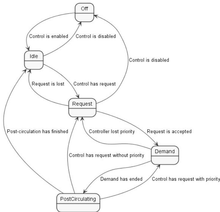
Dependent on the required functions of the appliance and connected sensors and components, several operation modes for Central Heating (CH) and Domestic Hot Water (DHW) can be selected, which are described hereafter.
