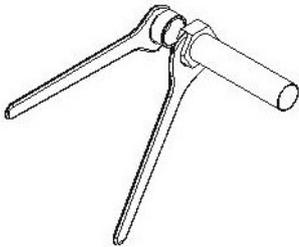
**DO NOT TIGHTEN FITTINGS WITHOUT SUPPORTING THE GAS PIPE, A BACKING WRENCH MUST BE USED.**
