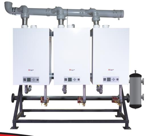
The Cascade System features multiple, high efficiency, fully modulating, low water content boilers, where off cycle losses are substantially reduced and dissipated heat from stored water is far less than a single large capacity boiler.
