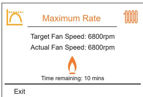
The boiler will run at Maximum Rate for 10mins as long as there is sufficient cooling load
