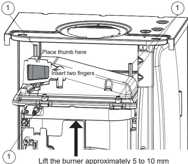
Lift the burner approximately 5 to 10 mm from the heat engine and then pull forward by the same amount.
