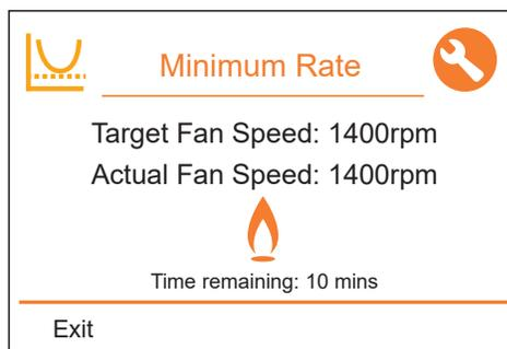
The boiler will run at Minimum Rate for 10mins
