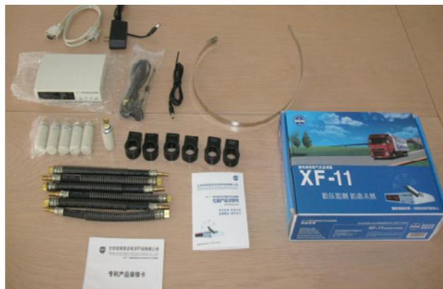
Tire Pressure Monitoring System Device
