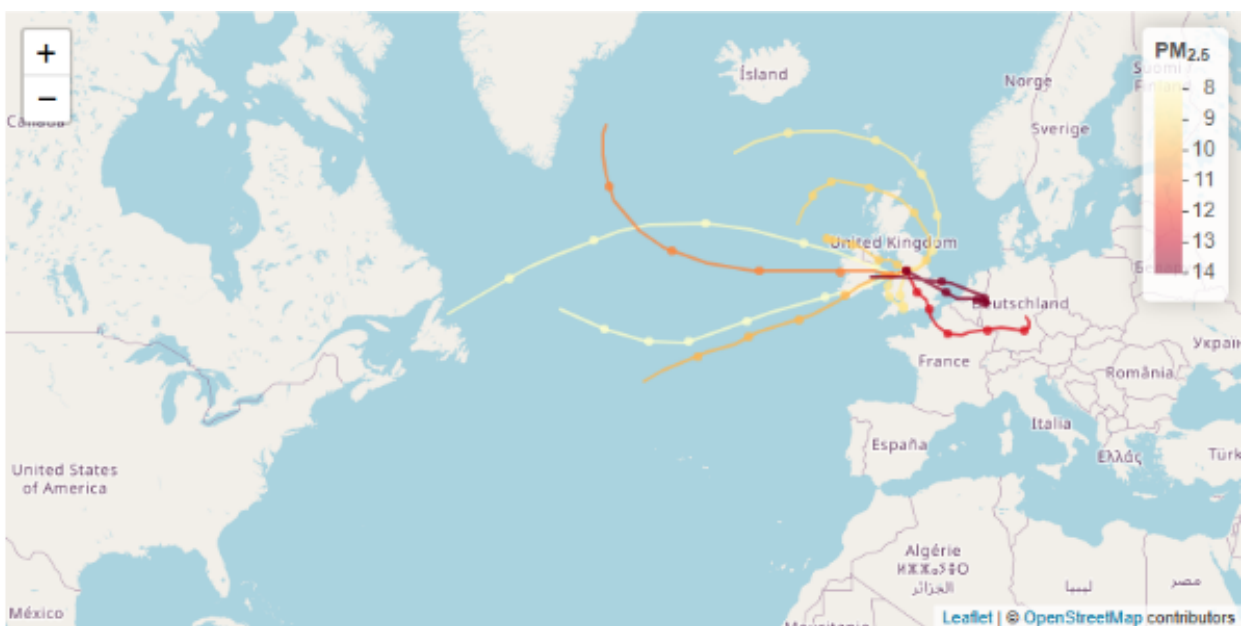
Figure C.2 - Example back trajectory plot for top ten highest daily PM 2.5 concentration, August 2025
