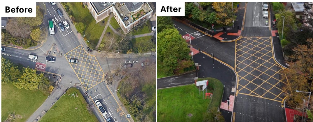
Figure 0-7 - Upgraded signals with added pedestrian phases, Higher Lane/Pinfold Lane, Bury (before and after junction improvement works)
