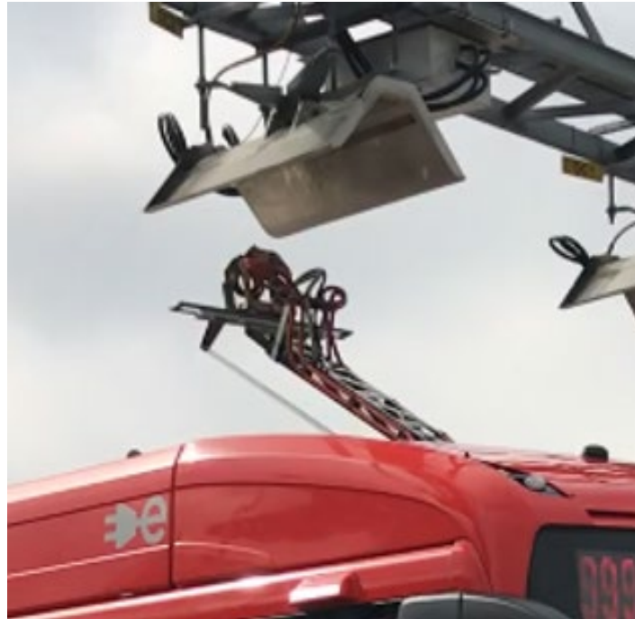
J-3105-2 Vehicle-mounted Pantograph Connection
