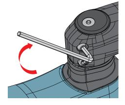
Torque the barstem to **5.2Nm**
