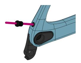
Route the rear derailleur Di2 cable through the chainstay.
