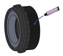
Apply a layer of good quality assembly paste to the threads of both bottom bracket cups. We recommend assembly paste from Morgan Blue (Auqaproof Paste) or r.s.p. (Creak Freak Assembling Paste).
