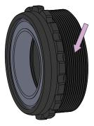
Clean the inside of the frame bottom bracket & the bottom bracket cups with an isopropyl alcohol.
