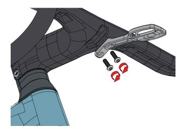
Install the computer mount and tighten the 2 bolts to **2 Nm.**
