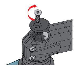
**4-13** Note that the notch on top cap sits in between the slot on the back of the barstem.
