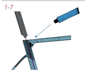
Apply Black Inc Installation Compound to the inside of the seat tube. Connect the Di2 cable to the battery. Insert seat post into the frame to the desired height.
