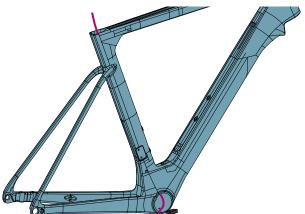
Route Di2 wire through seat tube and out through bottom bracket hole, attach Junction B to the end of the Di2 wire at the bottom bracket
