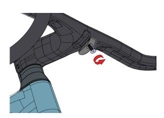
Release the bolt and remove the cover.
