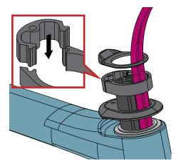
Assemble the appropriate top bearing cover, spacers and stem spacer.
