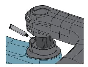
Apply assembly compound on the steerer tube and slide the barstem onto the fork steerer.
