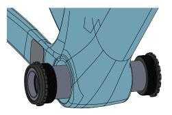
Thread the cups into the frame and torque the cups down to 30nm for the drive side and 40nm for the non drive side. We recommend using Park Tool BBT-47.
