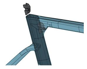
Insert the seat post clamp into the frame. Note: you may find it easier to keep this from falling down into the frame if you coat it in carbon prep compound, and/or tilt the frame downwards
