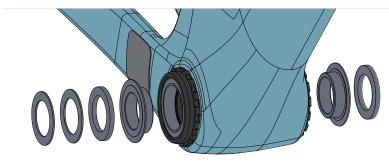
Drive Side 1mm+1mm+3mm+29mm reducer Non Drive Side 29mm reducer+3mm For Shimano Hollowtech II cranksets, install the included 24mm Wheels MFG reducers and spacer in the following sequence.
