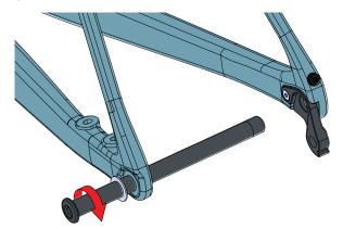
Remove the thru-axle and remove the hub. Install the rear wheel and tighten the thru-axle (with the nylon washer) to 12Nm.
