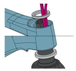
Assemble both top and bottom headset bearing and slide fork steerer, brake hose and Di2 wires through top bearing.
