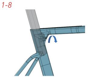
Secure the seat post by carefully tightening the grub screw to  $\bf 5.5\text{-}6Nm$
