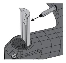
Insert anti-compression plug into the gap in front of the fork steerer and the apply assembly compound around it. **4-12** Install the top cap cover.
